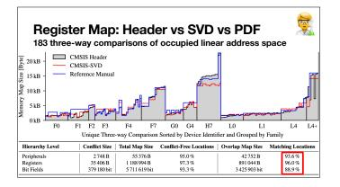
And finally we compared the register maps reconstructed form the CMSIS Header, vs the CMSIS-SVD vs the PDF.
